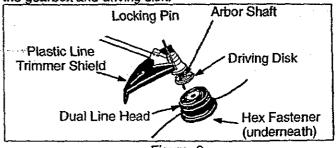
Figure 6 Locking Pin **Dual Cutting Head** Plastic Line Trimmer Shield Install Counterclockwise Remove Clockwise Blade Nut/Spark Plug Wrench
